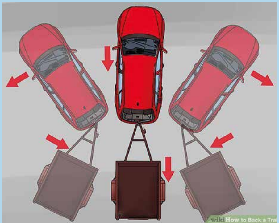
Backing 101: Turn your wheels opposite the desired turn to form an angle, but don't hold this too long as you start backing. Straighten front wheels and make small course corrections. That's it!
